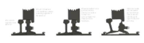
Diagram 1: Shows a switch point and stock rail. A wheel tread is shown on the left, and the gage side of the stock rail is on the right. The text indicates that the wheel tread cannot contact the gage side of the stock rail.
