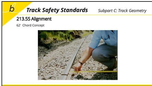
**Key Message:** Maintaining appropriate curve alignment helps reduce wear on the track structure and rolling stock and it is a critical component of derailment prevention.
