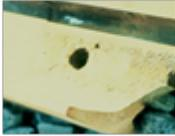
**Note:** Heat stress cracks in torch cut bolt hole.
